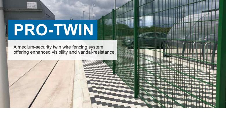
This Twin Wire Fencing System is a medium-security solution available in 656 or 868 mesh options. The 656 variant comprises twin 6mm horizontal wires and 5mm vertical wires, while the 868 option features twin 8mm horizontal wires and 6mm vertical wires.
